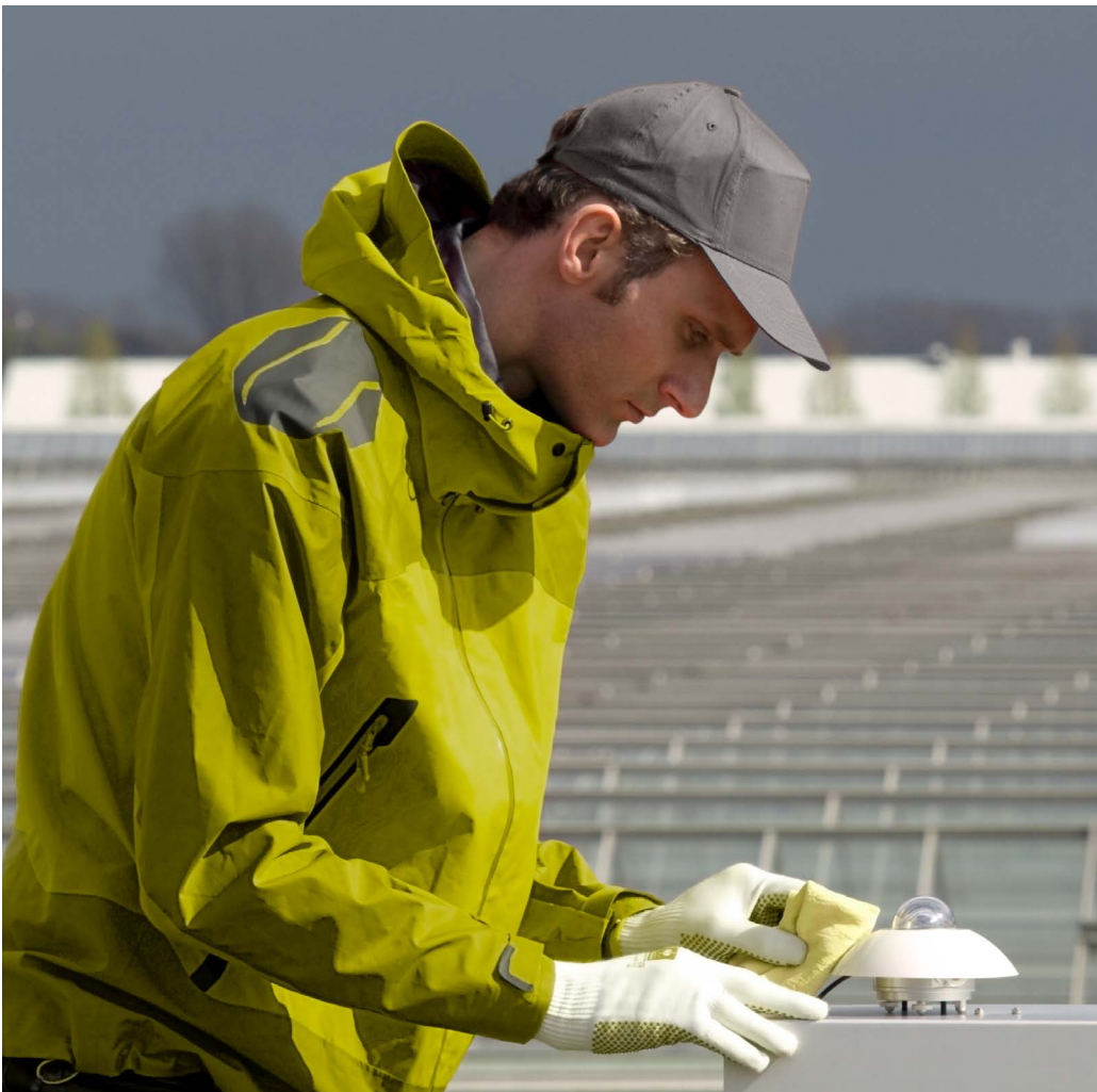
Figure 2 Application example: Solar sensor used for greenhouse climate control (pyrgeometers can also be used).
