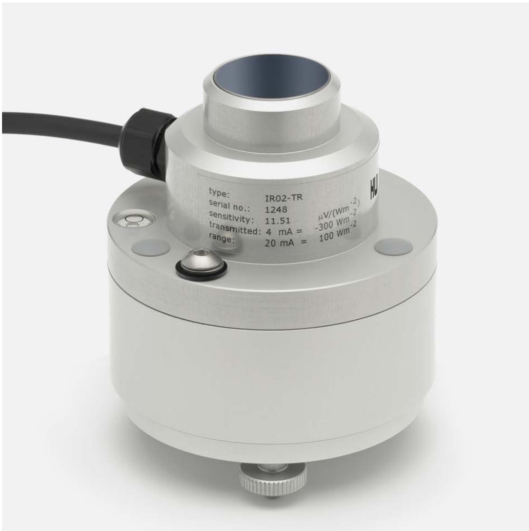
Figure 7.1: IR02-TR pyrgeometer with heater and 4–20 mA transmitter.
