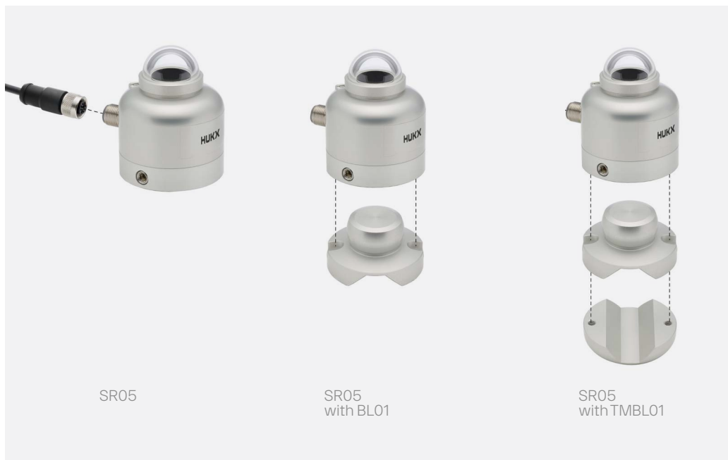
Figure 5.21 From left to right: SR05 in its standard configuration with 3 meter cable; with optional ball leveling for easy mounting and leveling on a (non-)horizontal surface; with optional ball leveling and tube mount for easy installation on a 25 to 40 mm diameter tube. Mounting bolts are included with the ball leveling and/or tube mount.
