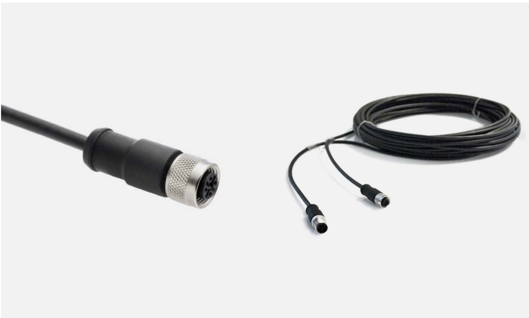
Figure 9.1: On the left the SR05 cable with M12-A female connector on sensor end. The cable is non-stripped on the other end. Its length is 3 meters standard and available in 10 and 20 meters too. On the right Hukx extension cable with connector pairs, with male and female M12-A connectors, available in 10 and 20 meters.
