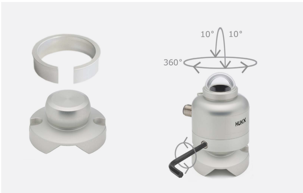
Figure 5.4.1 On the left SR05's ball leveling including shim (mounting bolts not displayed) and on the right SR05 placed on the ball leveling mount. Loosen the countersunk set screw on SR05's side to unlock, allowing placement of the ball head and SR05 leveling, and tighten it to lock the ball head mechanism. A 4 mm hex key is the only tool needed to place and remove the ball leveling and to allow and disallow leveling adjustment. The shim, included when ordering ball leveling, allows for smooth leveling and should be positioned properly in the center of the bottom plate of SR05.
